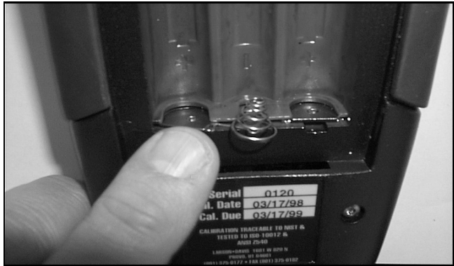
Figure 1-8 Battery Terminal Assembly orientation.
